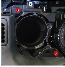
**8.** Pry the bottom kick panel off and remove the screw holding the speaker panel in place.
