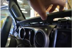
5. Remove the (4) screws holding the top of the gauge cluster panel and pry off.
