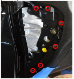
7. Now remove the (2) screws holding the top of the driver side speaker panel in place.
