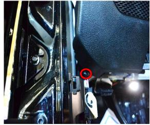
**9.** Then remove the two panels under the steering wheel to reveal the (3) remaining screws holding the speaker panel in place. Remove the remaining (3) screws.
