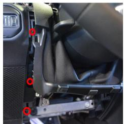
10. Pull the Speaker panel off and disconnect the light switch connector.
