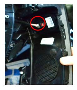
**11.Preparing the mount.** Align the SDHQ JL Switch Pros Mount to the speaker panel and mark the 4 holes dotted below to be drilled. Drill out holes with a 5/32" drill bit. Use a Dremel to cut out the rectangular portion in between the drilled holes.
