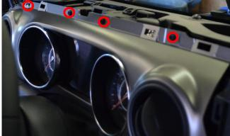
**6.** Now the driver side panel can be pried off revealing the (6) screws holding the speaker panel in place. Remove the (6) screws holding in the speaker panel.
