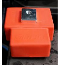
5. Take the positive fuse assembly and place it on top of the positive terminal, using the supplied 5/16" hex head bolt to tighten it down. Return the plastic terminal shield over the positive connection. Take the negative cable and place it onto the top terminal and tighten down using the supplied 5/16" hex head bolt. \*In our experience we have found that factory Panasonic batteries tend to have slightly smaller negative terminals than standard SAE specifications\*.
