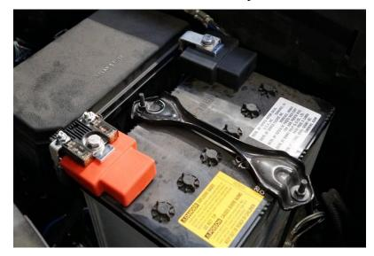
1. First remove the negative wire from the terminal by loosening the 13mm nut holding it down, being careful to not let it contact the positive terminal once removed. Then remove the plastic shield coving fuse assembly on the positive terminal and the 13mm nut holding the fuses to the terminal. Loosen both terminals using a 10mm wrench and remove them from the battery.
