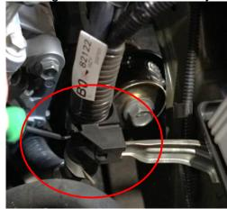
3. The positive fuse assembly has (2) tabs that need to be trimmed for proper electrical connection to the terminals, shown below. The fuse assembly can be separated from the connecting wires by removing the (2) nuts on the top. Replace the wires before moving forward with the installation. \*If you're not using the supplied battery boots then trimming this fuse assembly is not needed for proper connection.\*
