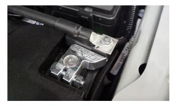
7. Connect all negative wires to the negative terminal. Enjoy your new SDHQ Built Ford Ranger Complete Billet Battery Terminal and Distribution Kit!
