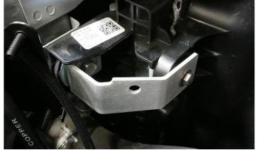
5. Next assemble your Billet Distribution Block using the provided hardware. Attach the 2 AWG negative wire to the block using the 3/8" eyelet. Using the M8 socket head bolt and flange head nut attach the block to the mount. Route the negative wire down under the engine side of the battery and positive wires to eventually come back up on the back side of the battery as shown.
