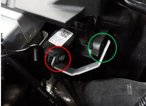
**4.** Adjust the mount to a desired position and replace the 10mm bolt with the supplied S.S. M6 hex head and tighten. Thread the 13mm bolt in the rest of the way to lock the mount in place.
