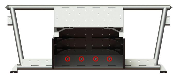
3. Align the Driver Side Plate next to the Front Plate and Main Plate. There is a total of (7) 5/16" – 18 x 3/4" Grade 8 Hex head bolts that will be used on this side. (3) bolts will connect the Driver Side Plate and the Front Plate. The other (4) bolts will connect the Driver Side Plate and the Main Plate. Use the 5/16" washers on both sides of the bolt.
