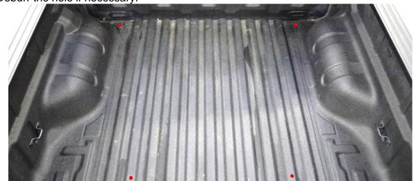
10. Install (1) 5/16" - 18 Rivet Nut into each front hole as shown below.
