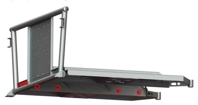
**5.** Align the Driver Support Tube with the Main Plate and Front Plate as pictured. Insert (4) 3/8" – 16 x 3/4" Grade 8 Hex head bolts with 3/8" washers through the Driver Support Tube on the Front Plate and Floor Plate. Place 3/8" washers and thread 3/8" – 16 Lock Nuts onto the 3/8" Hex head bolts. Repeat this for the Passenger Support Tube.
