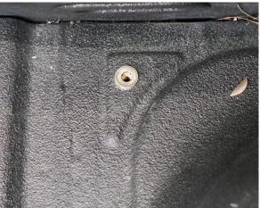
**11.** Align the bed rack back into position. Begin threading (1) 5/16" – 18 x 1" S.S. Countersunk bolt and (1) 5/16" Countersunk Delrin Washer into the front driver side mount. Repeat for the front passenger side mount. See pictures below. Do not fully tighten mounting hardware until all hardware is installed.
