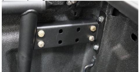
**14.** From underneath the truck bed, locate the rear driver mounting hole. Place (1) Capture Nut Plate flat against the truck bed with the weld nut facing the ground as shown below. Thread (1) 7/16" – 14 x 1" Bolt and Washer through the Bed Rack and bed into the Capture Nut Plate.
