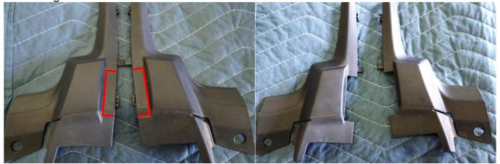
**11.** Install the cut cowls and press-in clips. Install lights using the hole, secure bigger lights with the slot if applicable. Position lights as desired. Enjoy your new SDHQ A-Pillar Light Mounts!
