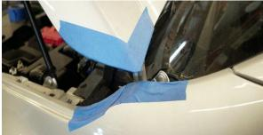
3. Using a flat head screw driver, remove the press-in clip arrowed to the right. Remove the cowl and set aside. (Passenger side shown)
