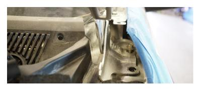
**5.** Now the driver side light mount can be placed into position. Follow the pictures below. Thread in both hood hinge bolts. Leave them loose for adjustments.
