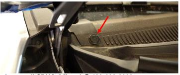
4. On the driver side, locate the hood hinge to fender bolts as shown right. With a 10mm wrench, loosen the rear bolt until there are only a few threads holding it on. Remove the front bolt completely. \*\*Mark the outline of your hood hinge before loosening the 10mm bolts. This will assist in alignment during installation\*\*
