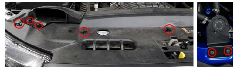
3. Position the Switch Pros Power Module over the SDHQ Mount and secure it using the Switch Pros supplied hardware.
