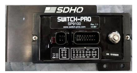
Connect the Switch Pros Power Module power cable and place the boot over the connection. Install (2) #10 – 24 clip on barrel nuts as shown below.
