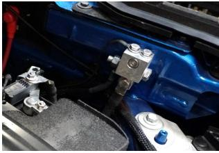
**5. Positive Terminal Install:** The factory power distribution bar will need to be removed from the cover. To do so, disconnect any wires connected to the distribution bar and remove from the vehicle. Using small flat head screw drivers or similar tools, pry each clip from the cover and remove the power distribution bar. Reconnect all wires to the power distribution bar as found.
