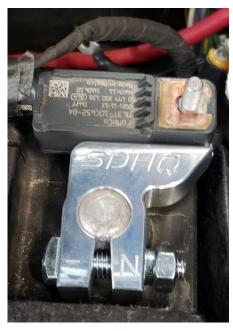
**4. Negative Distribution Block Install:** Remove the 12mm bolt securing the factory ground wire to the fender. Position the Negative Distribution Block and secure using supplied M8 Socket Head Bolt. Secure the factory ground wire to the 5/16" hole and attach any other accessories to the Negative Distribution Block.
