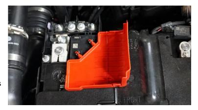
3. **TS1 Install.** Add the 5/16" battery bolt to the terminal and attach the TS1 Terminal to the BMS using the supplied stainless M6 flange head nut. Place the battery post washer on the negative terminal with the TS1 over it. Using a rubber mallet, tap the terminal to help it seat on the battery post. Tighten the 5/16" battery hardware once you're happy with terminal location. Leave grounds disconnected for now.
