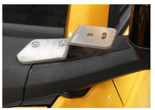
**4.** The supplied  $\frac{1}{4}$ " hardware is used for locking the driver to passenger rotation of lights such as Baja Designs XL80 and LP4 Series Lights. Place the bolt through the outer slot of the light mount with a light installed and tighten down at desired angle of light projection.
