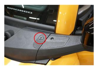
**3.** Place the mount on top of the cowl lining up the (2) bolt holes and loosely threading in the supplied M6 bolts and washers using the supplied T27 bit. Adjust the mount as desired and tighten down the bolts. Repeat steps 2-3 for the passenger side mount shown to the left.
