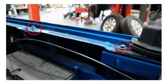
**3. Preparing your vehicle Continued.** Remove the (2) 10mm nuts holding down the driver side tie down. Remove the tie town and remove the 10mm fender bolt shown in green.
