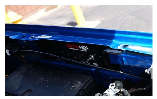
6. Installing the Power Module Mount Continued. Tighten the front 10mm fender bolt that's located under the driver tie down. Then place the tie down back on the vehicle and tighten the (2) 10mm removed in step 3. Replace the final 10mm fender bolt that helps hold the tie down and tighten. Enjoy your new SDHQ Built Power Module Mount. You can now proceed to wiring your Switch Pros.
