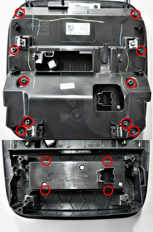
8. Install Switch Pros Keypad. Place the 3/16" acrylic backer into the hole formally occupied by the Upfitter switch block as shown and notice the 2 holes that are partially obstructed. Using your 5/32" drill bit, drill through the backer and clear the obstructed holes.
