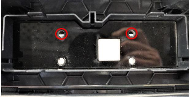
**9.** Mount your Switch Pros 9100 or RCR-12 in the SDHQ 3D Printed Keypad Mount and thread in the (4) #6-32 x 1" studs into the keypad (**Note:** The RCR-12 Keypad will only use the lower 4 holes for install as shown).
