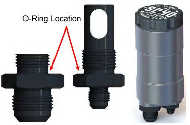
10. Lube the AN-6 Anti-Cavitation Fitting and AN-10/AN-12 Fitting. Install the AN-12 Push Lok 90° Fitting onto the AN-12 Flare. Install the AN-6 Push Lok 90° Fitting onto the AN-6 Fitting. Angle these fittings such that the factory hoses will connect without any kinks in the hose. Tighten all fittings.
