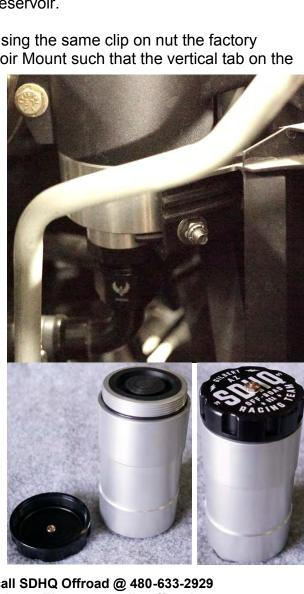
9. Locate the AN-6 Anti-Cavitation Fitting and the AN-10 Flare Fitting. Check for the O-rings on these fittings, arrowed in red on the right. Lube the threads of the AN-6 Anti-Cavitation Fitting with assembly lube. Thread this fitting into the right hole on the bottom of the Power Steering Reservoir where the SDHQ Logo is legible on the Cap. Lube the threads on the AN-10 Flare and thread this fitting into the other threaded hole. Tighten both fittings.
