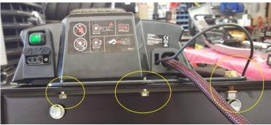
**10.** Tighten the 3/8" bolt first, then evenly snug down the (3) 6mm bolts to approx. 7 ft-lbs.
