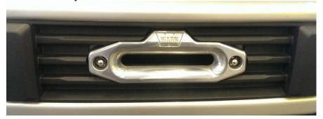
Center the Winch mounting holes on the plastic insert. The mounting holes will be 10" apart, centered on the middle horizontal rib. The tall top edge will be lined up with the top inner edge as pictured. Mark the center of the holes and drill out to 7/16" starting with a small pilot bit.
