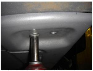
3. Removing the bumper. Remove the (2) 10mm bolts holding the plastic valance to the upper portion of the bumper. Remove the (4) 21mm nuts holding the bumper on, and remove the bumper.
