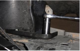
**4.** Remove the front skid plate brackets and factory tow hooks by removing the (6) 15mm bolts mounting them.
