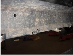
2. Remove the 3 push clips holding the rubber dust guard on. Remove the (6) 15mm bolts holding the factory skid plate on. Remove the skid plate.
