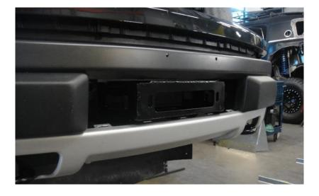
**10.** Using the first holes you drilled in the frame as a guide, drill (2) more 5/8" holes through the bumper.
