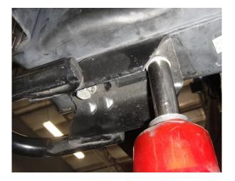
**5.** Install the Winch Mount between the factory tow hooks and the frame using the factory hardware. Install so bends raise the plate up, and the brace is toward the rear of the truck. Use the rear set of slotted holes (narrower set) to install.
