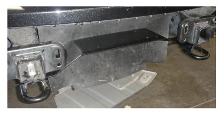
6. Bolt the Fairlead Mount to the underside of the Winch Mount using the 2 outer bolts only.
