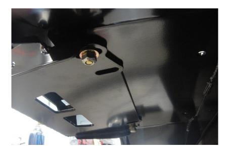
7. Drill a 5/8" hole on each side of the frame through the lower slotted hole of the Fairlead Mount.
