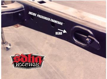
**2.** Align holes in bracket with the outside frame rail oval ports. The bolt holes should be towards the upper portion of the oval frame ports, and the SDHQ bracket should sit flush against the bottom of the Ford frame rail. Install (2) 1/2" x 13 grade 8 bolts with a drop of thread locker and torque to 100 ft lbs.
