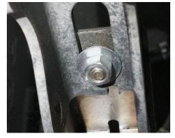
**4.** Check alignment of the driver shock eye to the lower mount hole, lifting the vehicle if the shock eye is low and lowering the vehicle if it is too high. Once aligned slide the shock guard up and replace the factory hardware with the supplied M12 bolts and nuts, threading them on loosely.
