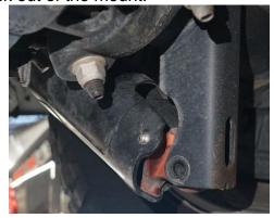
**3.** Align the shock guard onto the lower mount and loosely thread the supplied 3/8" bolt through slot on the mount using the 1" washer on the inside of the mount as shown.
