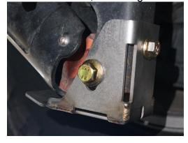
**5.** Repeat steps 2-4 for the other shock and tighten all 3/8" hardware. Lower the vehicle down to ride height and tighten the lower shock bolts to factory torque specs. Enjoy your new SDHQ Built Raptor Shock Guards!
