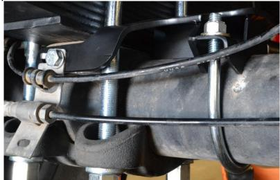
**4.** Repeat steps 2-3 for the passenger side. Be sure to place the ABS/parking cable bracket on the outside of the spring perch when installing the passenger Bump Pad.
