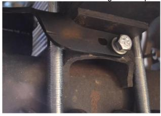
**3.** Place the U-bolt under the axle and install into the Bump Pad using the 3/8" lock nut and 3/8" washer. Torque to 25 ft-lbs or until the pad is in full contact with the axle, **BUT DO NOT OVER TIGHTEN**. Torque the M8 hardware to 25 ft-lbs.
