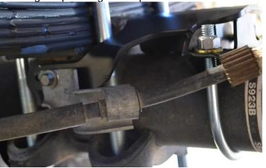
**5. Installing U-Bolt Plates.** Align the U-Bolt Plate holes with the Deaver leaf spring center pins before installing the U-Bolts. Bolt the U-Bolts once the U-Bolt Plates are set properly as pictured below.
