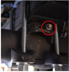
2. Align one of the Bump Pads on the driver side perch. Bump Pads are not directional. Install (1) M8-1.25 bolt and M8 washer set on the front and (1) set on the rear of the Bump Pad, leaving loose for now. Be sure to place the brake bracket back when installing the Bump Pad.
