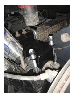
**3.** Lower the truck back down to the ground. Tighten all bolts including the leaf spring bolts. Torque the Deaver Leaf Spring U-Bolts to yield. Tighten the  $\frac{1}{2}$ " – 20 U-Bolts until the pad is in full contact with the axle, **BUT DO NOT OVER TIGHTEN**.
