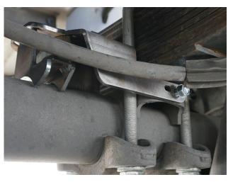
**3.** Place the U-bolt under the axle and install into the Bump Pad using the 3/8" lock nut and 3/8" washer. Torque to 25 ft-lbs or until the pad is in full contact with the axle, **BUT DO NOT OVER TIGHTEN**. Torque the M8 hardware to 25 ft-lbs.
