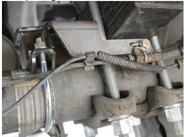
**5. Installing U-Bolt Plates.** Align the U-Bolt Plate holes with the leaf spring center pins before installing the U-Bolts. Bolt the U-Bolts once the U-Bolt Plates are set properly as pictured below.
