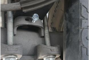
**2.** Align one of the Bump Pads on the driver side perch. Bump Pads are not directional. Install (1) M8-1.25 bolt and 5/16 washer on the front replacing the brake line bracket on the outside of the mount. Use the supplied 5/16" bolt on the rear of the Bump Pad. Leave both loose for U-bolt installation.
