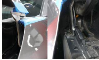
**6.** Next locate the Driver Side Support Bracket, carefully slip the bracket behind the light mount so that the open slot slides over the removed fender bolt hole and install the supplied M6 Button Head bolt and washer. Insert the ¼" hardware and loosely bolt the A-pillar to the Support Bracket. Apply Anti-Seize Lubricant to the stainless steel button head hardware and install through the light mount and support bracket slots with washers and nylock nut.
