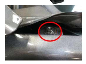
**4.** Remove the 13mm head bolts that holds down the back of the hood hinges to the truck.
