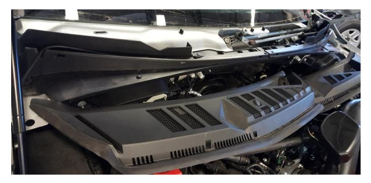
**5.** Loosen the 10mm head bolt that was covered by the cowl at the top of the fender, but do not remove, leave threaded in.
