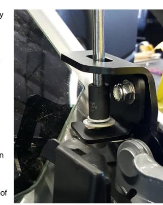
\*\*\*Double check all hardware is installed correctly and tight\*\*\*
