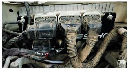
6. Tighten down the bolts that hold the Power Module Mount. Place the wire back on top of the bolt and tighten the nut back down. Now the wiring can be ran.
