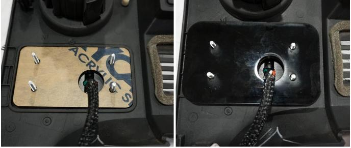
5. Proceed with wiring your Switch Pros. Finally, install the radio center bezel with all electrical connectors and the gauge cluster bezel. Enjoy your new SDHQ Built Switch Pros Keypad Mount!
