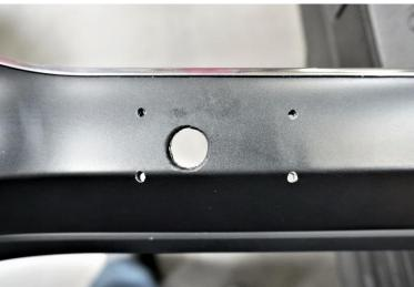
**4.** Install your Switch Pros keypad into the mount and align over your holes on the drilled panel. Feed the wire harness through the larger hole and thread in the (2) 9/16" button head bolts into their holes as shown on Page 4. Use the (2) 1" button head bolts with backers to finish attaching the keypad, note that Backer 2 will be placed in the lower hole, closest to the front of the panel.
