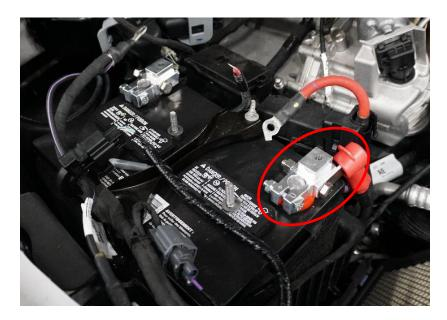
7. Install the intake in the reverse order of Step 2. You have completed the SDHQ Ford Super Duty Battery Terminal Upgrade! \*\*\*Double check all hardware is installed correctly and tight\*\*\*
