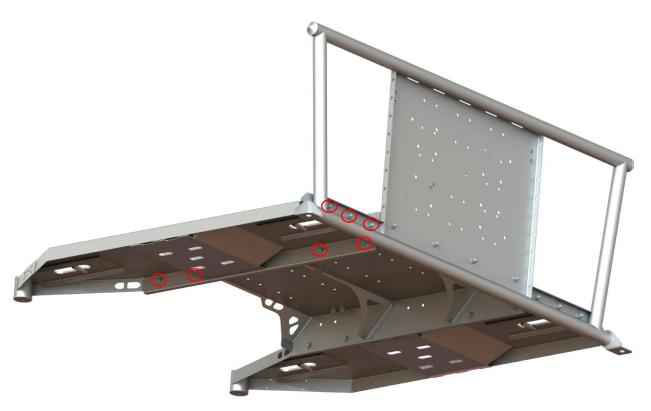
**5.** Align the Driver Support Tube with the Floor Plate and Front Plate as pictured. Insert (4) 3/8" – 16 x 3/4" Grade 8 Hex head bolts with 3/8" washers through the Driver Support Tube on the Front Plate and Floor Plate. Place 3/8" washers and thread 3/8" – 16 Lock Nuts onto the 3/8" Hex head bolts. Repeat this for the Passenger Support Tube.
