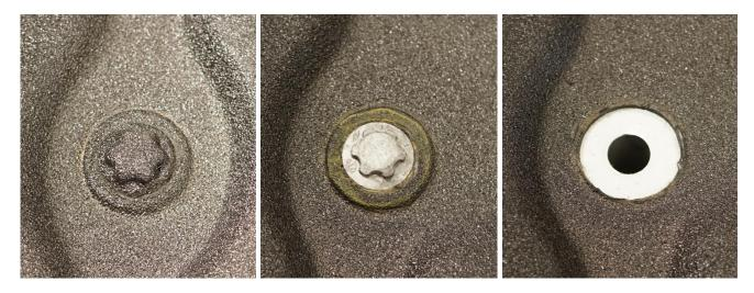
9. Use a Torx Plus EP-24 bit to remove these bolts. Align the Bed Rack mounting holes over the bolt holes in the bed. Tighten the bed bolts by hand first using the EP-24 bit starting with the (2) bed bolts at the rear of the truck. Torque to 60 ft lbs. Install the (2) Plastic Round Tube Plugs into the mounting tubes.
