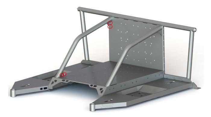
**6.** Use (2) 5/16" – 18 x <sup>3</sup>/<sub>4</sub>" Grade 8 Hex head bolts, (4) 5/16" washers and (2) 5/16 – 18 Lock Nuts for each tie down mount. Bolt the mounts as pictured below. The mounts can be placed where needed on the Bed rack.
