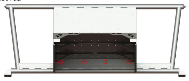
3. Align the Driver Side Plate next to the Front Plate and Floor Plate. There is a total of (7) 5/16" – 18 x ¾" Grade 8 Hex head bolts that will be used on this side. (3) bolts will connect the Driver Side Plate and the Front Plate. The other (4) bolts will connect the Driver Side Plate and the Floor Plate. Be sure to use the 5/16" washers on both sides of the bolt.
