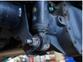
**3.** Align the shock guard onto the lower mount and replace the shock bolt with the supplied M14 flange head bolt and nut. Leave the bolt loose to allow the shock guard to be adjusted.
