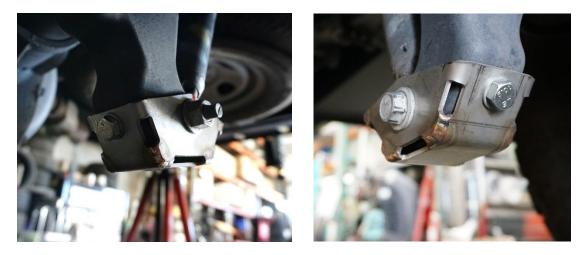
5. Repeat steps 2-4 for the other shock and tighten all M10 hardware. Lower the vehicle down to ride height and tighten the lower shock bolts to factory torque specs. Enjoy your new SDHQ Built Super Duty Shock Guards!
