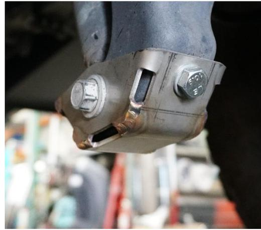
5. Repeat steps 2-4 for the other shock and tighten all M10 hardware. Lower the vehicle down to ride height and tighten the lower shock bolts to factory torque specs. Enjoy your new SDHQ Built Super Duty Shock Guards!
