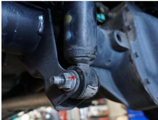
3. Align the shock guard onto the lower mount and replace the shock bolt with the supplied M14 flange head bolt and nut. Leave the bolt loose to allow the shock guard to be adjusted.
