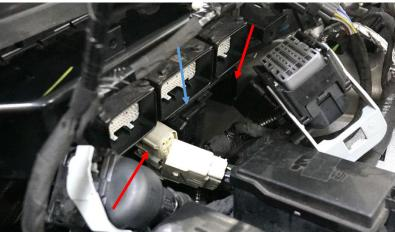
**5.** You are ready to remove the plastic cover now. There are (6) clips securing the plastic cover to the fire wall, (2) on top and bottom, (1) on both sides. Start on the passenger side and work your way towards the engine. Once unclipped, the fuse boxes and connectors will need to be adjusted such the plastic cover can be removed. Re-install all connections and fuse boxes.
