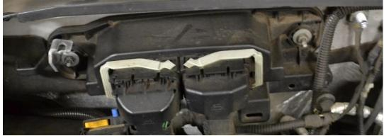
**8.** Installing the Power Module to the SDHQ Mount. Align the Switch Pros Power Module to the SDHQ Mount. Insert the Switch Pros Supplied bolts through the Power Module and Mount. Secure using the #8 S.S. SAE Washers supplied in this kit and the Switch Pros supplied nut. Use the diagrams shown below to align the Switch Pros Power Module.
