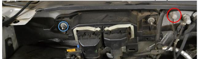
**7.** Slide the SDHQ Power Module Mount Bracket behind the PCM nut loosened in Step 6. Tighten this nut until the bracket doesn't fall. This will be tightened in a later step.
