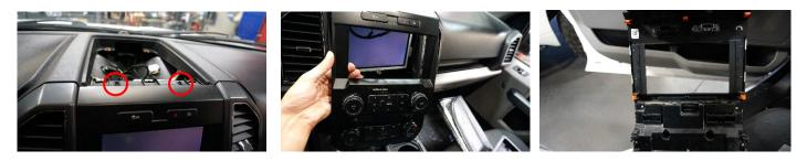
**5.** Remove the lower radio bezel by removing the (2) screws using a 7mm socket. If equipped with a Bench seat skip to Step 8.
