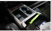
7. Remove the left dash air vent trim, there may be electrical connectors on the panel so be careful when removing. Remove the coin holder from the panel and set the panel aside.
