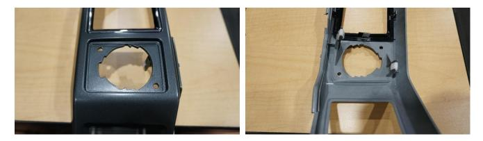
8. Install the Switch Pro into the Keypad mount and use the supplied button head bolts to attach the keypad to the mount. Install the Keypad mount onto the panel using the supplied Thread Forming Screws through the factory panel holes.
