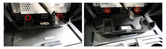
6. If equipped with a Center Console, remove the Flow Through panel using plastic trim tools release the rear of the panel under the center console lid. Then pull back on the trim to remove it from the console.
