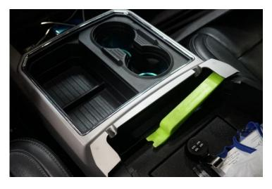
4. If your F250+ truck is equipped with LED lit cup holders and wireless phone charging, there will be two LED lights in the cup holders and another connector under the trim panel that will need to be removed before the panel can be taken from the truck. If your truck does not have these options or has others, proceed carefully and make note of where connectors are located for your panel.
