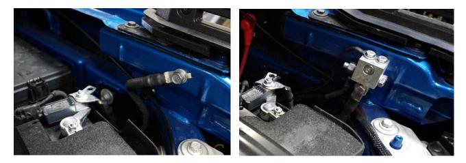
**3. Positive Terminal Install:** The factory power distribution bar will need to be removed from the cover. To do so, disconnect any wires connected to the distribution bar and remove from the vehicle. Using small flat head screw drivers or similar tools, pry each clip from the cover and remove the power distribution bar. Reconnect all wires to the power distribution bar as found.
