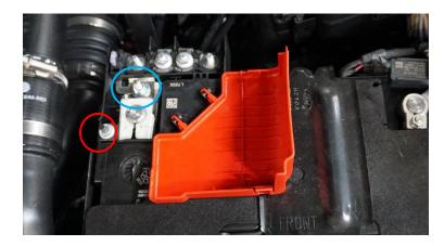
2. Negative Distribution Block Install: Remove the 12mm bolt securing the factory ground wire to the fender. Position the Negative Distribution Block and secure using supplied M8 Socket Head Bolt. Secure the factory ground wire to the 5/16" hole and attach any other accessories to the Negative Distribution Block.
