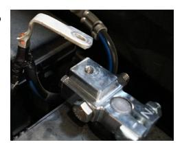
**5.** With the terminal installed, finish wiring any accessories to the negative terminal and tighten all hardware.
