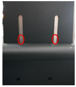
**6.** Disassemble everything and drill the (4) holes on your Pro Eagle Jack Mount. (**Note:** When drilling stainless steel Pro Eagle Jack Mount, drill bits will have a tendency to "walk" off of the center of your marked hole, it is recommended to drill your holes oversized to minimize the need to redrill)
