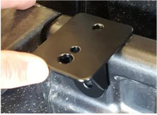
**2.** Mark the top and side holes on the bed. Drill a 7/16" hole where marked, and clean hole from any burrs.
