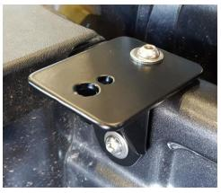
5. Use the appropriate hole for the light you are using. Mount and wire up your light.
