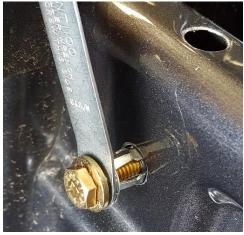
4. Mount the chase light bracket so the flat plate is on top, and the 2 holes together are facing the rear. Use the (2) ¼"-20 x 1" stainless steel button head bolts and washer to mount, use the anti-seize on all stainless hardware.
