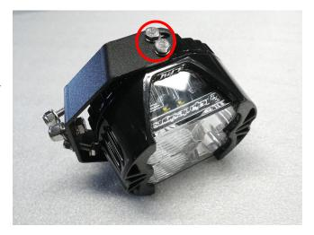
3. Place the blinder on top of the mount and rethread the (2) bolts back into the light housing, note that the notch must be at the bottom next to the light bracket. Adjust the light to the desired angle and tighten down the bolts to 5ft-lbs.
