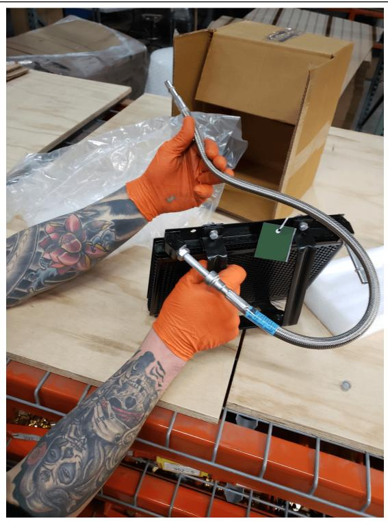
3. 1 of the 2 Long Lines should have a female fitting on one end and another female fitting on the other end. This line is intended to connect the fuel cooler to the engine.
