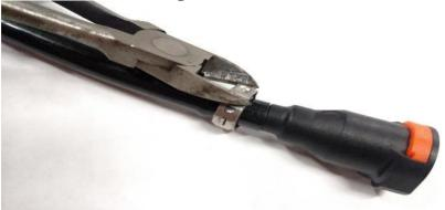
6. Using pliers, squeeze the tab in the middle of clamp.
