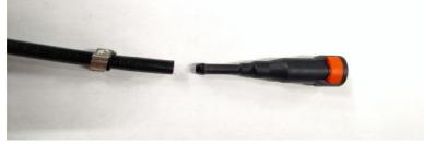
3. With the supplied female quick disconnect fitting and fuel line clamp, slide the clamp over your factory nylon fuel line.
