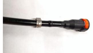
4. Insert the quick disconnect fitting into the nylon.
