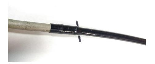
1. Identify the factory nylon fuel lines under the vehicle. The factory nylon line is molded to the hardline. Looking at the line, there will be a noticeable dimple in the line like shown in photo above.
