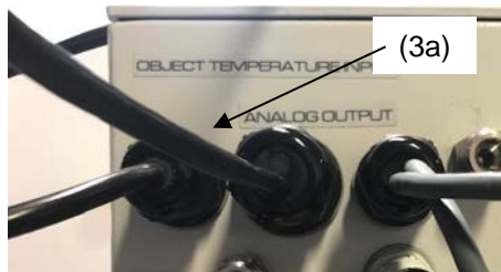
Figure 30: Connection cable on the "Object temperature input" connection (3a)
