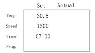
Note: To prevent from misoperation, if 10 minutes no action since pause, device will stop working and power off automatically.
