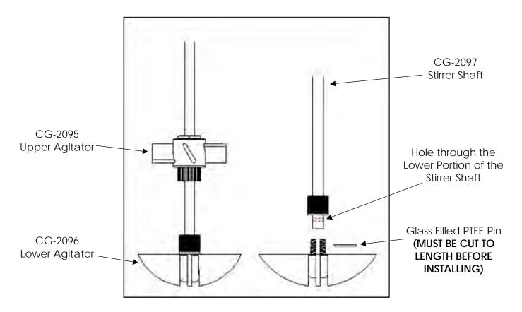
The stirrer shaft and agitators are assembled and installed when shipped. Use the following instructions should you need to remove or adjust these components.
