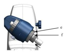
**Note:** Prior to commissioning, hand-tighten the plastic screw nut (f)
