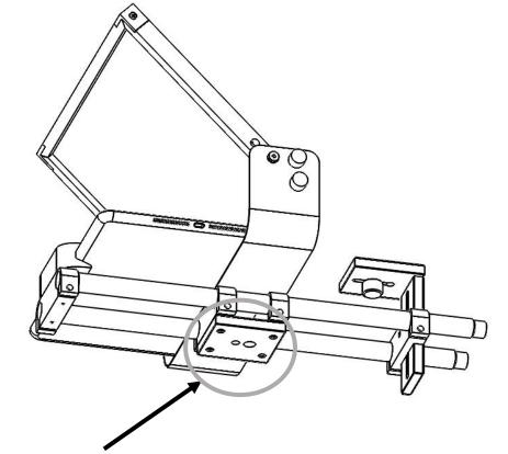
The TMP 500 features ¼-20 and 3/8-16 mounting holes for tripods.
