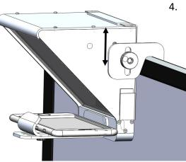
Using the thumb screws on the side holders, center the hole in the cover with your computer's camera.
