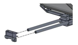
Slide the Camera Plate onto the rails on the opposite side of the Beam Splitter.
