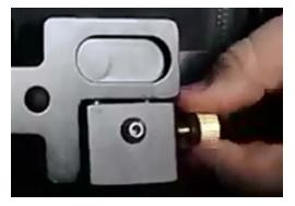
Tighten the safety screw to fix the control arm in the arm seat on your preferred side to keep the control arm from slipping out during operation.
