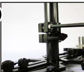
26. We have two ways adjust this alignment. The first and simplest method is to loosen the adjustment knob on the Telescoping Clamp and rotate the parts until they are aligned as seen in image #27; then, just tightening the adjustment knob back. Keep the 1" of Telescoping Post visible below the Telescoping Clamp as before.
