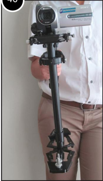
40. Once you're done adjusting the side-to-side balance, you might have to go back and tweak the front-to-back balance in order to get a true, fine balance of the entire system. You can either just do a visual check to judge for the correct horizontal balance of your GLIDE GEAR DNA-5050 or employ a lightweight bubble level (not included) to make sure.
