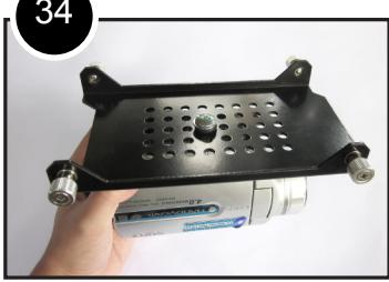
**NOTE: Do not over tighten this screw. Doing so will likely damage the threaded insert in your camera base.**
