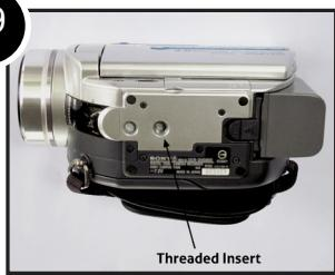
29. Check the bottom of your camera and locate the threaded insert.
