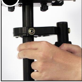
45. As you handle your GLIDE GEAR DNA-5050, you will want to use your Guide Hand to lightly hold onto either the point just under the yoke and bearing assembly as seen in image #45, or a spot down by the Base Platform as seen in image #52. When using your GLIDE GEAR DNA-5050, these two areas allow for the easiest and best control. Again, the hand position you pick will depend on the type of shots you need to take.
