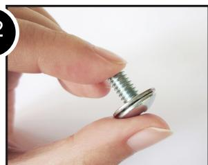
32. Use a camera mounting screw and a  $\frac{1}{4}$ " washer to attach the Camera Plate to your camera.
