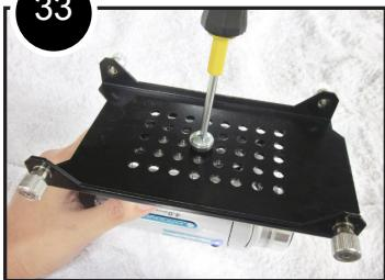
33. Place your camera on your lap or better yet, on a stable but cushioned surface—a folded towel on a table is a good example. Now that the Camera Plate is in position, use a screwdriver to affix the Camera Plate to your camera with the camera mounting screw and the  $\frac{1}{4}$ " washer pair.
