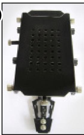
27. Another way of correctly aligning said parts is to use an Allen wrench to loosen the screw on the top part of the Telescoping Clamp as shown in image #26. Do this until you can rotate and correctly align the parts as shown in image #27; remember to retighten the screw.
