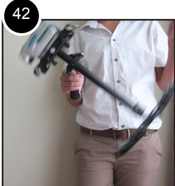
42. Once more, if the vertical balance is properly set, you will be able to move about quickly as well as start or stop moving suddenly and still keep the Central Post vertical. To adjust the GLIDE GEAR DNA-5050's vertical balance you can either attach or take out Counterweights from the Base Platform, or telescope the Base Platform in or out. When you have more or less the right amount of weight on the Base Platform, you can fine-tune the vertical balance further by using the Telescoping Post.
