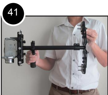
In short, if your GLIDE GEAR DNA-5050 is vertically balanced, your camera will remain level and the Central Post will stay vertical unless intentionally positioned otherwise. A vertically unbalanced GLIDE GEAR DNA-5050 will swing about and pendulum when you walk, run, or turn.
