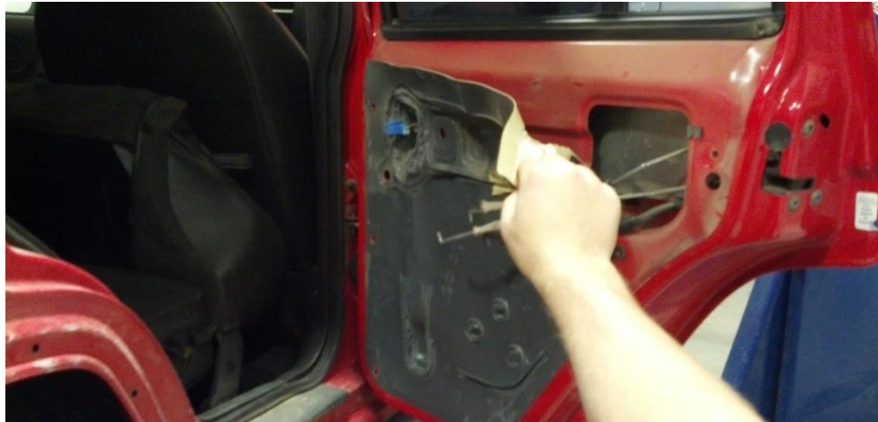
Figure 13 - Shows passenger side door after panel has been removed and liner has been partially pulled away.
