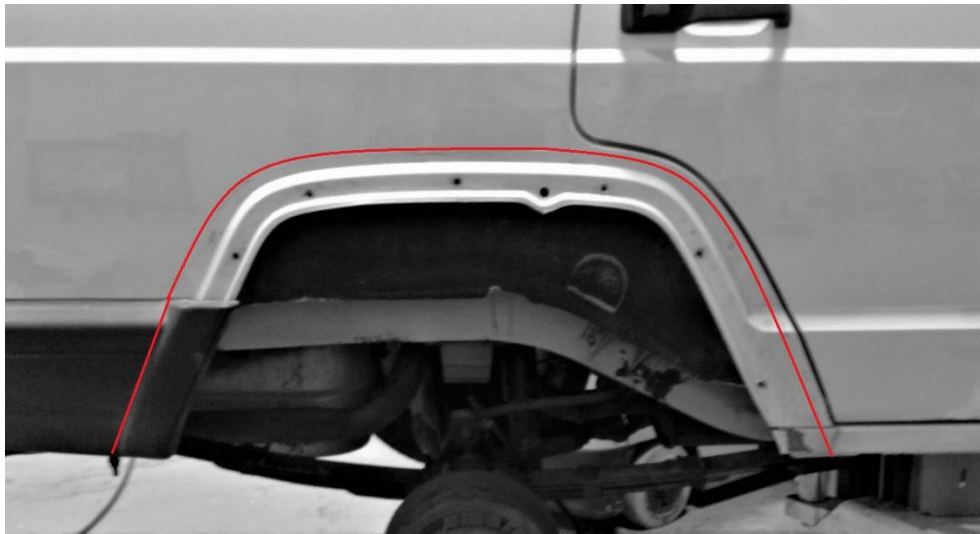
Figure 17 - APPROXIMATE trim line/scribe line for rear wheel well (Passenger side shown)
