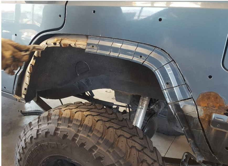
Figure 20 - Driver side fender, partial outer fender piece removal
