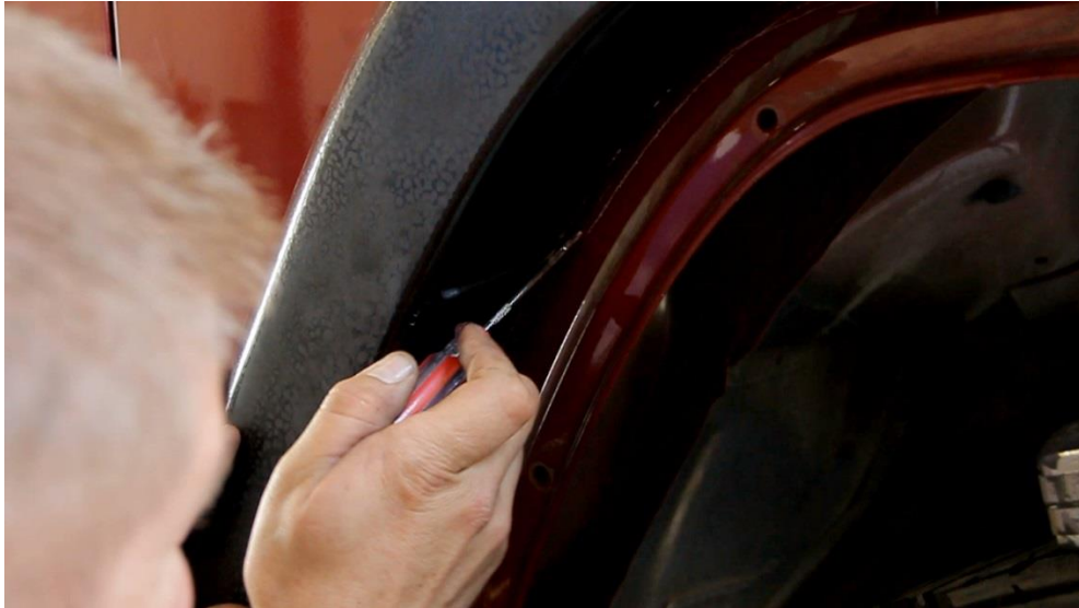
Figure 5 – Making the scribe mark on front passenger's side fender
