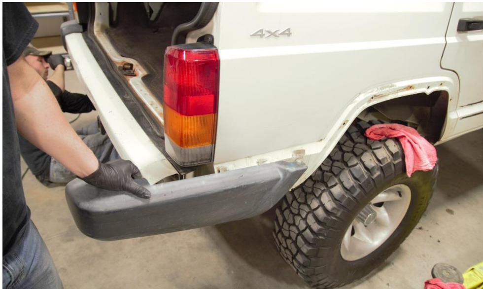
Figure 8 - Passenger side bumperette being removed.
