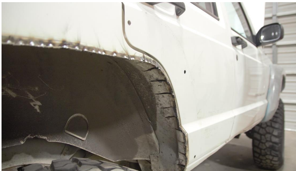
Figure 234 - Rear passenger side after welding and excess metal has been trimmed.
