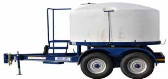
16 inch high speed truck tires & leaf spring suspension
